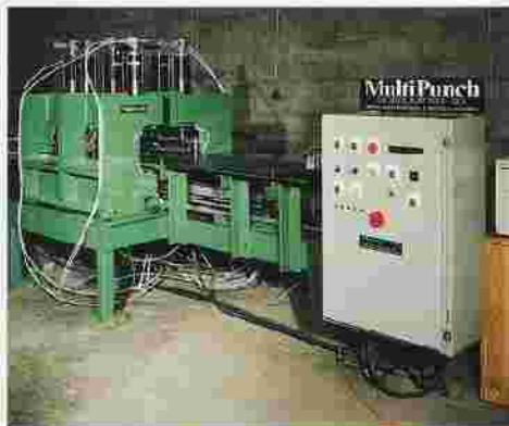
MultiPunch - 100 tons of programmable punching power
